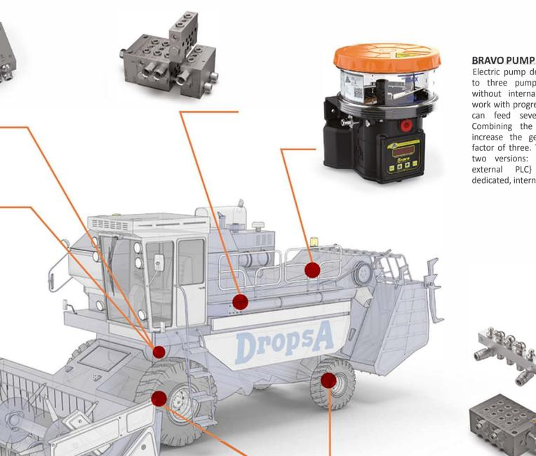
Electric pump designed to work with up to three pumping elements, with or without internal by-pass. Designed to work with progressive dividers, this pump can feed several independent lines. Combining the pumping outputs will increase the generated flow up to a factor of three. This pump is available in two versions: manual (controlled by external PLC} or automatic with dedicated, internal control system.
