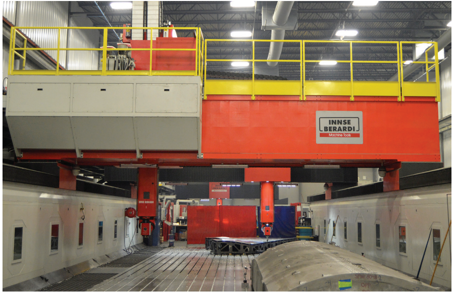
This Innse Berardi contour milling machine has a machining envelope of 975"×273"×117".
