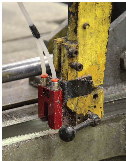
The challenge in developing MQL was in getting it to be easily adapted to all kinds of cutting equipment, said DropsA's Jason Craft. Here, an external MQL system has been added to a bandsaw at Visioneering.
