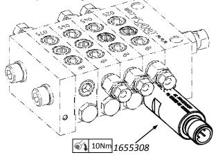
B) Visual monitoring pin with colour strip. This must be ordered with the divider element.
