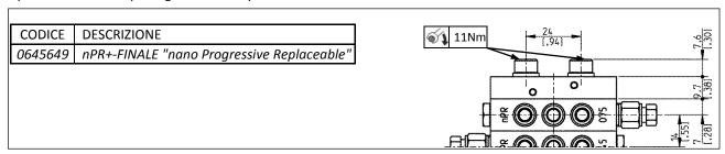
You can order the components of dividers block separately. Remember that washers and assemblies screws must be ordered separately also.
