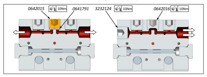
It is also possible to combine the flow rates of a metering element with the next metering element in the assembly by selecting an appropriate bridge metering element.
