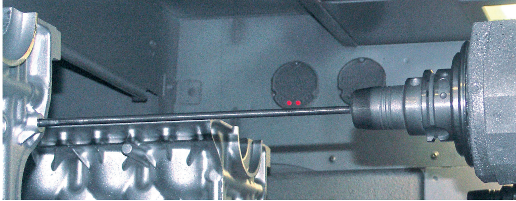
Deep hole drilling is, in particular, an application area of the MQL 2-channel technology.
