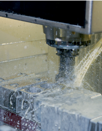
Example of Flood Coolant for cooling and lubricating when mechanically machining components.
